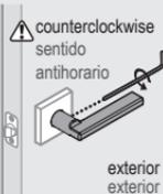
**B** Push up on lever base while tightening screws to keep latch horizontal and centered.
