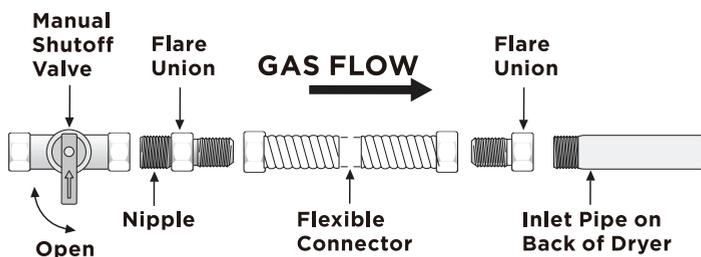
**All connections must be wrench-tightened**
