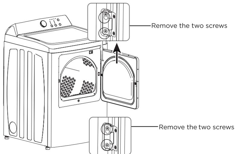
3. Remove the screws for the latch cover on the right side of the dryer and the screws for the locker cover on the left side of the dryer.
