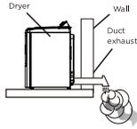
Use a 4" (10.2 cm) diameter rigid metal duct. Tape all joints, including at the dryer. Never use lint-trapping screws.
