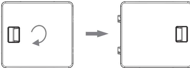
9. Align the hinges on the door with the hinge screw holes on the front of your dryer, then secure the door with the four screws you previously removed.
