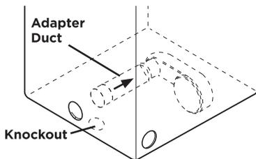
3. Insert the 4 inches (10.2cm) elbow through the rear opening and attach it onto the adapter duct.
