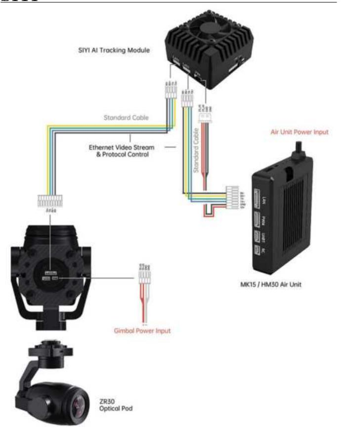
4. Please refer to the picture below to connect SIYI gimbal camera with flight controller and integrate attitude data.
