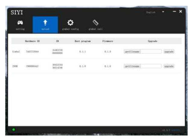
4. If the firmware is not latest, then click the "Select File" button in the "Gimbal" to import the latest firmware. And click "Upgrade" and wait till it is "100%" finished.
