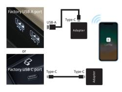
**NOTE!** The adapter should be plugged into the USB port that is for wired Apple CarPlay connecting if there are multi USB ports in your car.
