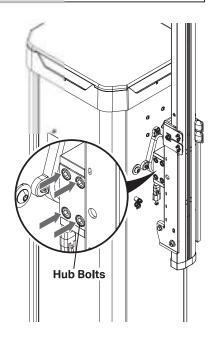
**NOTE:** If Limit Switch on the Hub is triggered please see appendix for instructions on how to reset it. Ensure the springs are in the correct orientation for the arm direction and begin setting limits. Start with the arm in the vertical/up position.
