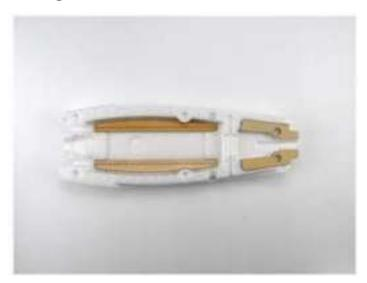
3. Apply foam glue to the bottom fueslage and bond the upper and bottom fuselage.
