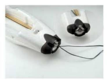
6. Adhere the front and rear ventilation covers. (If you have installed a GPS flight controller, please adhere the front ventilation cover after installing the GPS.)
