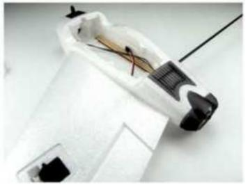
4. Install the front of wing-let. Open Box 3 and find the front of wing-let, apply glue to mounting position and appropriate pressure to let it bond firmly. Repeat for the Other Side. **Note**: the left and right wing-let are different.
