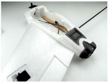
4. Install the front of wing-let. Open Box 3 and find the front of wing-let, apply glue to mounting position and appropriate pressure to let it bond firmly. Repeat for the Other Side. **Note**: the left and right wing-let are different.
