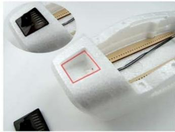
7. Adhere fuselage and the hatch cover. **Note**: please ensure that the corresponding South (S) and North (N) poles are aligned correctly.
