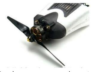
Based on your power requirements, select a 5 or 6-inch propeller. This product uses a pusher configuration, so install the propeller with the side that has text facing forward.
