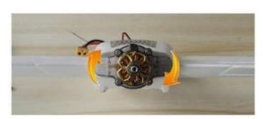
When facing motor, it should clockwise rotation, if not, please change either 2 of connector line.
