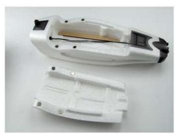
8. Install the handle on the hatch cover.
