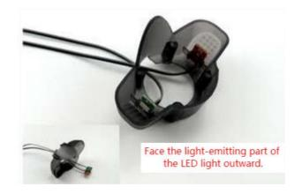
5. Install the motor mount by applying a circle of glue around the edge of the mount, 1~2mm from the edge. Also apply some glue on the wider upper edge. Then, install the mount onto the rear of the plane. After the glue has dried, rethread the wires of the led light through.
