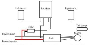
This is taking FUTABA receiver as an example.Left servo connect to CH1,right servo connect to CH6,ESC connect to CH3, UBEC and tail lamp can connect to rest any channel
