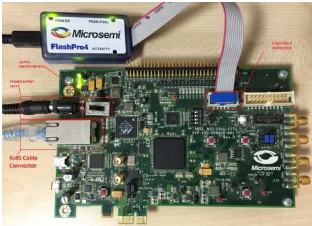
Figure 7 • SmartFusion2 Security Evaluation Kit Setup
