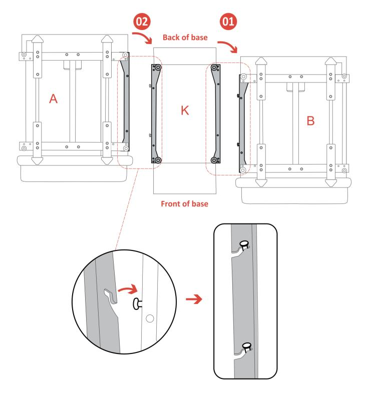
3. Once the holes on both frames are aligned, insert the cylindrical pin to secure the storage console and the right base.
