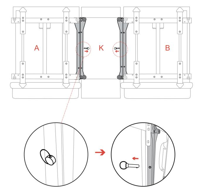
3. Lift the left base slightly upward and slide the two notches on the left base frame out of the protrusions to disassemble the left base.
