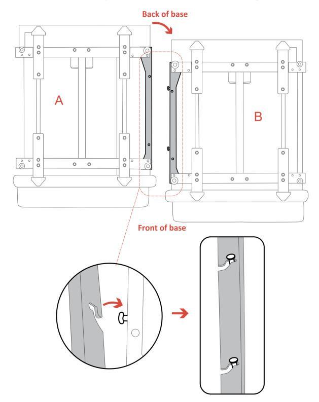
3. Once the holes on both frames are aligned, insert the cylindrical pin to secure the two bases.
