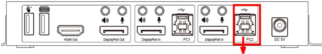
Disconnect the PC USB port and PC2 port connection
