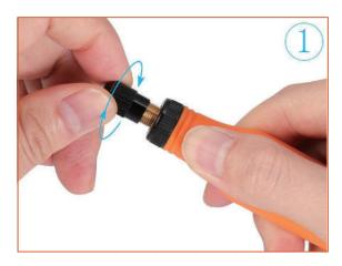
1. Press down the spindle locking 2. Choose the suitable collet button and unscrew the nut
