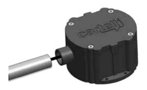
After pulling cable through plastic conduit, insert conduit inside slip joint on "puck." DO NOT GLUE (to un-install later, if needed).
