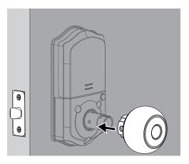
Tighten the screw with a screwdriver.
