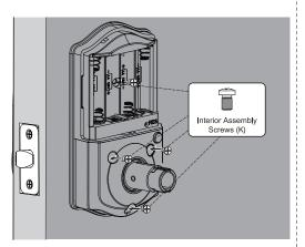
Insert 4 AA Alkaline batteries and put on the Battery Cover.
