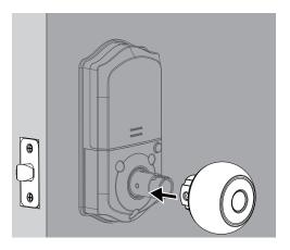
Tighten the screw with a screwdriver.
