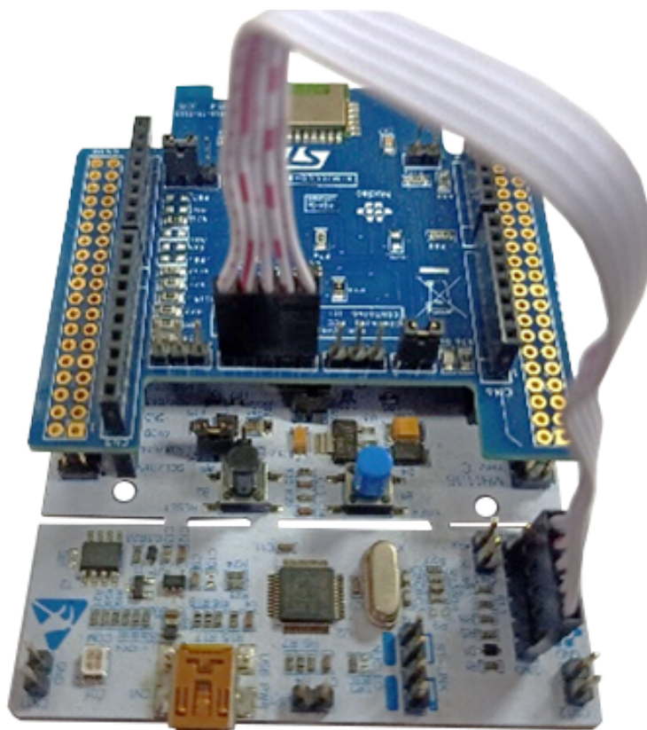
Figure 2. X-NUCLEO-BNRG2A1 and NUCLEO-L476RG connection via ST-LINK programming cable
