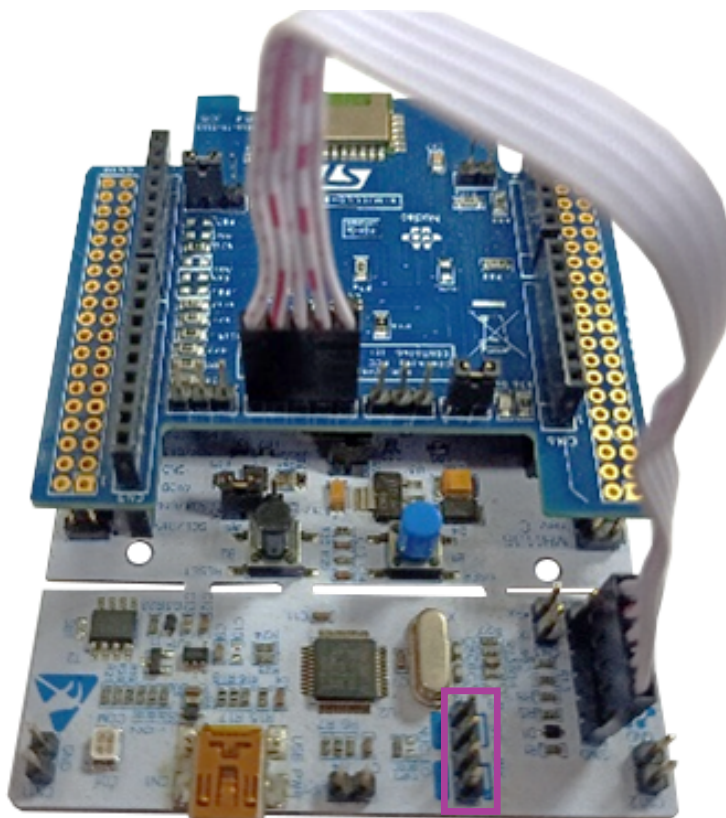
Figure 3. NUCLEO-L476RG development board CN2 pin (highlighted in purple)
