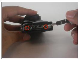
Unscrew the six 3.5mm Philips head from the outer casing.
