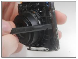
Pry the center casing off the camera. This is best done by separating the top and side sections individually.
