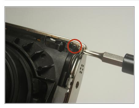
Unscrew the 3.5 mm Phillips head screw from the corner of the camera.
