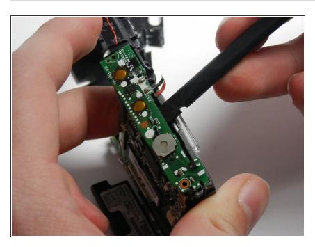
Pry off the top circuit board using the spudger.
