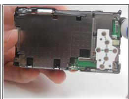
Unscrew the two 3.5 mm Phillips head screws in the metal plate.
