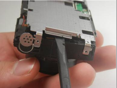
Pry the metal plate out using the spudger.
