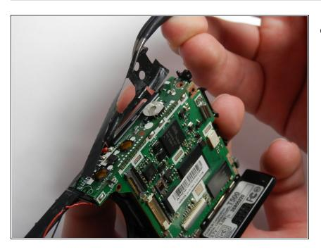
Use tweezers to pull back the plastic covering the top of the camera.
