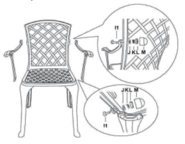
3.Attach the two arms (C1)to the back using stud (I1) washer (J), spring washer(K),nut(L),nut cap(M). Attach the two arms to the seat using stud (I1) washer (J),spring washer(K),nut(L),nut cap(M).
