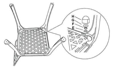
2.Attach the four legs (D1)to the seat using using washer (E), spring washer(F),nut(G),nut cap(H).
