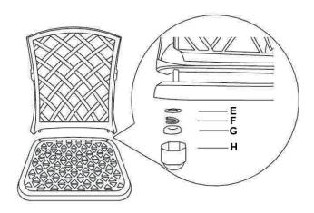
1.Assemble the back (A1) to the seat (B1)on an even soft clean surface using washer (E),spring washer(F),nut(G),nut cap(H).
