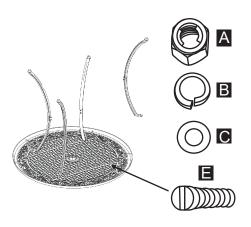
Turn over the table top.Attach the Stud M8(E) into the Nuts(inside table),Then,Attach table Legs(2) to the Studs on the Table Top (1) using Wahers and Nuts (A,B,C).DO NOT over tighten
