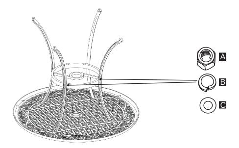
Attach the Table legs Support (3)to the four Legs (2)using flat washer,spring washer and nuts(A,B,C) DO NOT over tighten.
