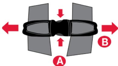
4. **Release** the buckle and place the harness straps to the side.
