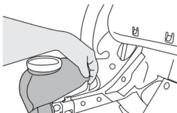
2. **Pull** over the cup holders so that the cover tucks under the cup holders.
