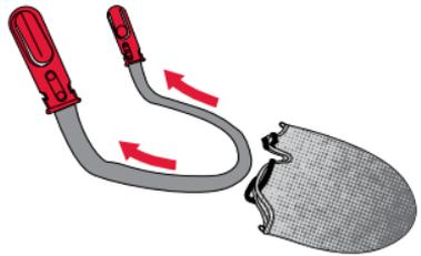
2. **Attach** the small elastic loops to the plastic tabs.
