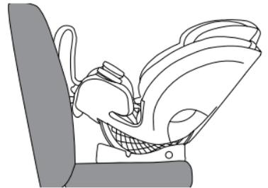
2. **Recline** child restraint to the appropriate position. Refer to page 14 to determine appropriate recline position.
