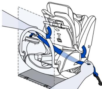
8. **Firmly press** the lower connectors **onto** their adjacent lower anchors.
