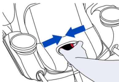
5. **Route** the lap vehicle seat belt through the **REAR**-facing belt path marked by blue labels.
