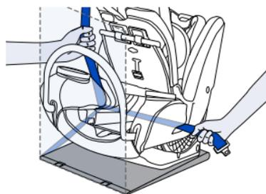
6. **Ensure** the belt is not twisted, then buckle the vehicle seat belt.
