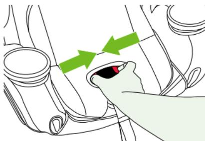
7. **Route** the vehicle lap-shoulder belt through the **FORWARD**-facing belt path marked by green labels.
