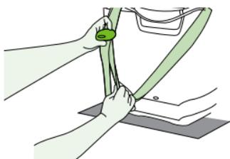
2. **Unhook** the top tether hook from the back of the child restraint and place it up and over the seatback.
