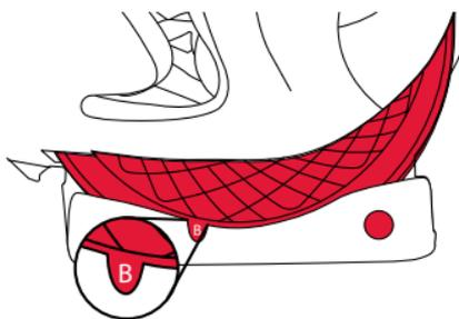
3. **Open** the CLICKTIGHT. **Squeeze** the CLICKTIGHT release buttons underneath the front cover flap and lift to open.
