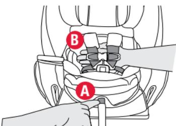
**NOTE:** Make sure enough harness adjuster strap is left hanging from the front of the seat. Use the inner slot as a reference point to measure how much harness strap can be left hanging from the front of the seat.
