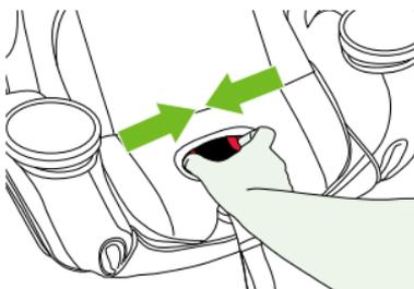
7. **Route** the lap vehicle belt through the **FORWARD**-facing belt path marked by green labels.
