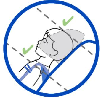
**IMPORTANT:** The provided lower infant insert **MUST** be used for children weighing 10 kg (22 lbs) or less in a rear-facing position. Do not use with a child weighing more than 10 kg (22 lbs) or in a forward-facing position.
