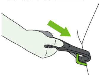
11. **Ensure** the connector strap is not twisted. Pull the end of the lower connector strap to remove slack.
