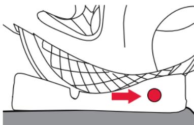
3. **Ensure** that no more than 7.5 cm (3 in) of the base hangs over front edge of the vehicle seat.
