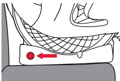
4. **Place** the child restraint **FORWARD**-facing on the vehicle seat so that the car seat base is flat on the vehicle seat and is parallel to vehicle seat.
