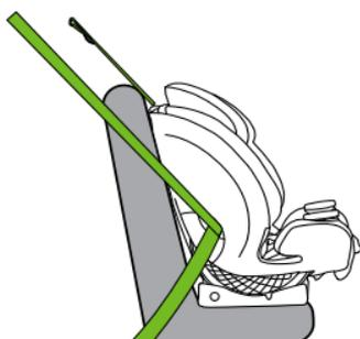
13. **Pull** the loose tether strap end to remove slack and secure excess webbing with the elastic band attached.
