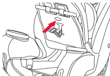
6. **Route** the buckle strap through the desired seat cover and slots, reaching on the other side of the open to pull the metal bracket through completely.
