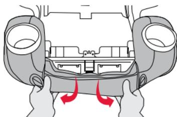
4. **Attach** elastics to the hooks on the shell.
