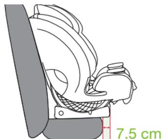
5. **Ensure** that no more than 7.5 cm (3 in) of the base hangs over the front edge of the vehicle seat.
