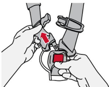
2. **Open** the CLICKTIGHT. **Squeeze** the CLICKTIGHT release buttons underneath the front cover flap and lift to open.
