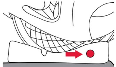
3. **Ensure** that no more than 7.5 cm (3 in) of base hangs over front edge of vehicle seat.
