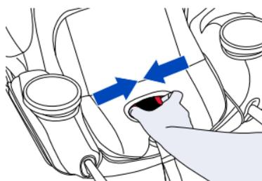
5. **Route** the vehicle lap-shoulder belt through the **REAR**-facing belt path marked by blue labels.
