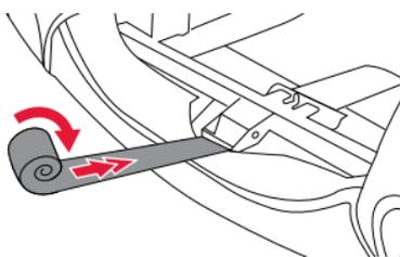
17. **Tuck** the remaining harness adjuster strap into the front of the cover.
