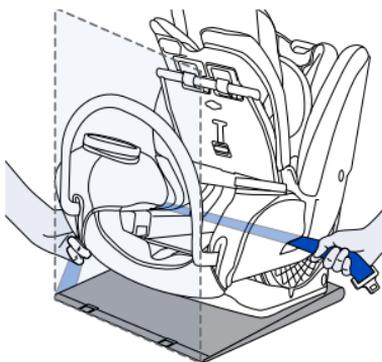
6. **Ensure** the belt is not twisted then buckle the vehicle seat belt.
