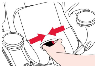
4. **Open** the storage pocket. **Remove** the lower connectors by pressing the spring tab, pushing the connector back while rotating down and forward off the anchor point.
