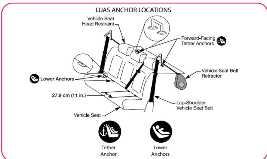
The Lower Universal Anchorage System or LUAS, is a system available on this child restraint that offers an alternative to vehicle seat belt installation methods. The figure above shows typical locations for lower anchors and tether anchors in a vehicle. See pages 2-3 for LUAS components on this child restraint.
