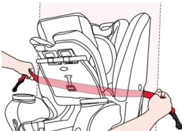
9. **Ensure** the connector strap is not twisted and remove slack.
