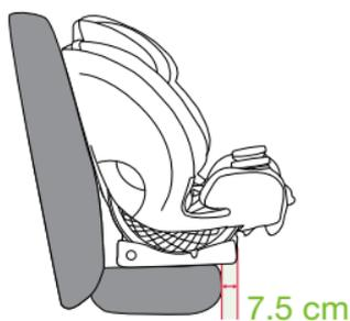
5. **Ensure** that no more than 7.5 cm (3 in) of the base hangs over the front edge of the vehicle seat.
