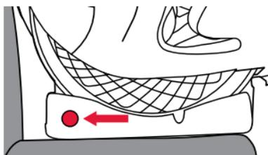
4. **Place** child restraint **FORWARD**-facing on the vehicle seat so that the car seat base is flat on the vehicle seat and is parallel to vehicle seat.
