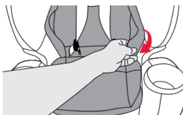
7. **Fold** the top of the seat pan cover with the vented side over. Position the harness straps behind the seat pan cover.
