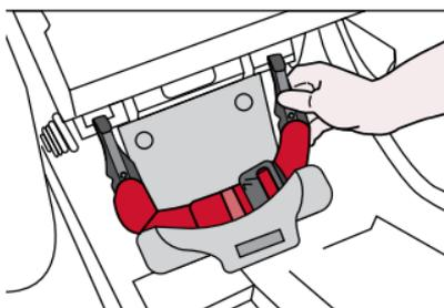
5. **Extend** lower connector strap to its longest length by pressing the grey button on adjuster.
