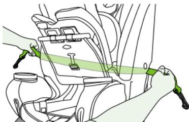
10. **Firmly press** lower connectors **onto** their adjacent lower anchors.
