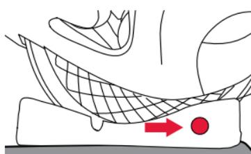
6. **Ensure** that no more than 7.5 cm (3 in) of the base hangs over the front edge of the vehicle seat.
