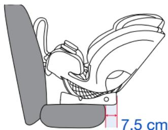
7. **Slide** the lower connector strap into the **REAR**-facing belt path marked by blue labels.
