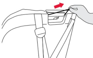
4. **Open** fasteners in headrest cover and pull cover away from the child restraint.
