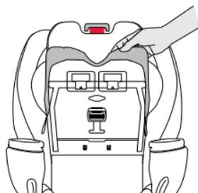
3. **Undo** the fasteners near the bottom of the harness straps.
