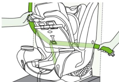
8. **Ensure** the belt is not twisted, then buckle the vehicle seat belt.
