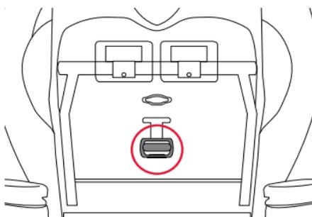
5. **Turn** the metal bracket sideways and push it up through the slot in the CLICKTIGHT and the slot in the seat cover.
