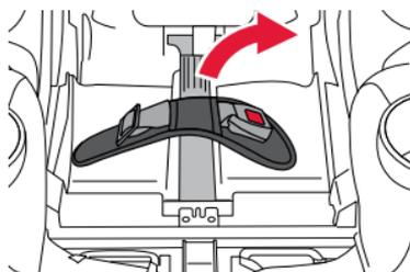
11. **Install** the buckle by turning its metal bracket sideways and routing it through the desired seat cover and slot in the CLICKTIGHT. Refer to adjusting buckle position page 12.
