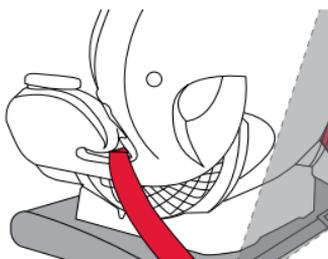
7. **Ensure** the shoulder part lays across the center of the child's chest, above the child's shoulder and does not contact the child's neck (A). The lap part of the vehicle belt is routed low across the child's upper thighs (B).
