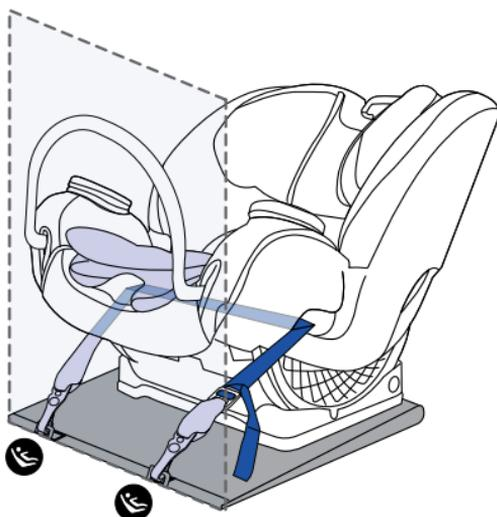
**NOTE:** Do NOT install by this method for a child weighing more than 13.6 kg (30 lb).
