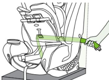
8. **Ensure** the belt is not twisted and fasten the seat belt.
