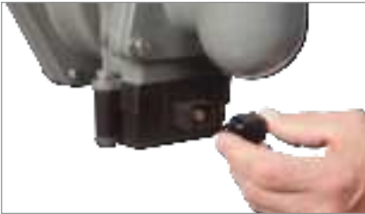
1. Remove the dust cover from the sensor.
