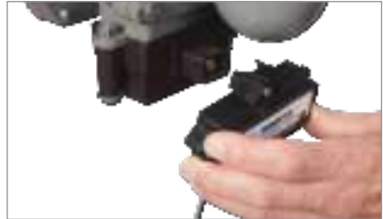
2. Press the activation module onto the sensor.
