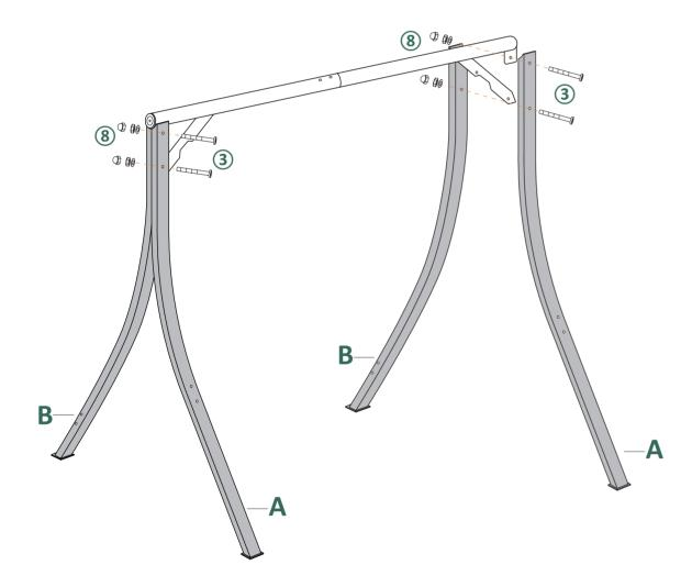
(3). Fix Leg Support #E between #A and #B with bolts #4 and nuts #9.
