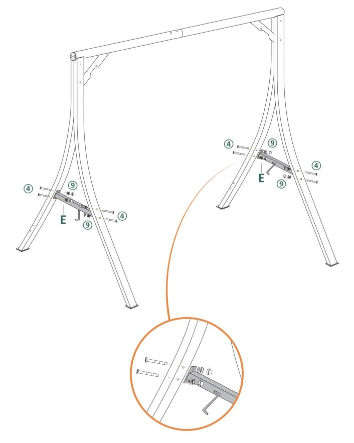
(4). Attach Bottom Support (Right) #F and Bottom Support (Left) #F1 with bolts #1 and nuts #9.
