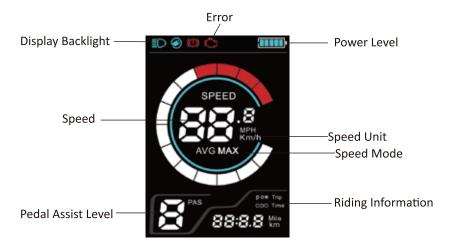
SPEED MODE: Average speed (AVG SPEED), maximum speed (MAX SPEED), real-time speed (RT SPEED).
