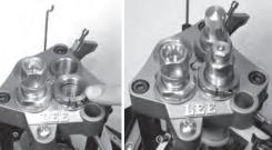
• Install bullet seating die and feeder assembly into position 3.
