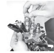
Die attach plate should be mounted at the 11 o'clock position. This will place action rod in a vertical position.
