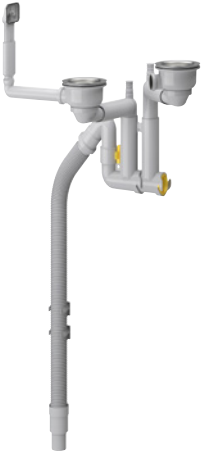
LILLVIKEN water trap/strainer 2 bowls. Water trap with connection for both dishwasher and washing machine. Polypropylene plastic. 103.254.28 900.-
