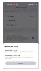
c. PTZ control direction flip: After you install the camera, if the camera direction is reversed, you can set the PTZ direction flip. After setting, the PTZ control will rotate in the opposite direction.
