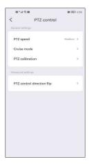
a. PTZ speed: If you think the camera rotates too fast, you can adjust speed to low at which the camera moves.
