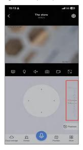
You can adjust the numbers to realize the digital zoom of the camera. 4X is the dividing line. (For WS02 Model)
