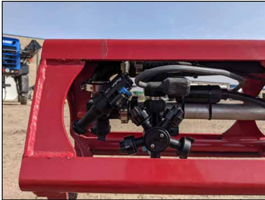
FIGURE 20. Example Plumbing for Boom Tip for 135'/20" 7-Section Boom
