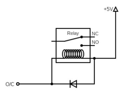
Please note that the maximum permitted voltage on the Open Collector contact is **5.5V** and the maximum current that can be sunk into the contact is **100mA**.
