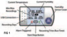
Current Temperature – The current temperature reading Current Humidity – The current humidity reading Min/Max Recordings – The minimum and maximum temperatures that have occurred since the device was initialized.
