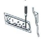
3. If necessary, use the strap (6) to secure the back of the unit in place. The strap (6) can be bent by band to the desired angle.
