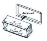
2. Band the tabs of the mounting sleeve (1) outward into the dashboard for a secure mounting.
