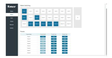
① **Matrix:** You can click and select an output (1~16) firstly, and then select an input source (1~8). One route of video output configuration is completed. You can switch it freely.
