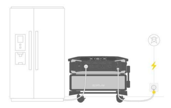
UPS (Uninterruptible Power Supply) is a device or a system that provides continual power supply and protects your appliances from damage if the incoming power is interrupted.
