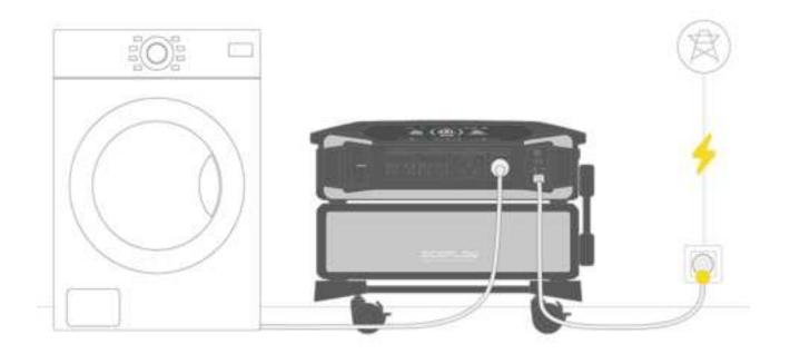
X-Fusion is an advanced technology that ensures all AC output sockets provide optimal output when the product is in bypass mode (when you recharge and discharge the device simultaneously, the device enables bypass mode automatically), in terms of wattage and amp. In the fast charging mode, the output will always be 7.2kW no matter how much the input is.
