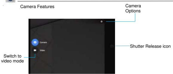
Switch - A switch between Camera to Video. Shutter Release - For taking picture. All other option available by clicking the gearhead icon are listed in the table below.
