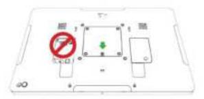
Plug Elo power-over-ethemet (POE) adaptor into recess, ensuring connector on bottom of adaptor lines up with connector on back of the I-Series 2.0.
