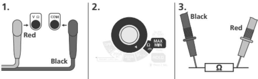
1. Connect the red test prod to the V  $\Omega$  input socket (12) and the black test prod to the COM input socket (8).
