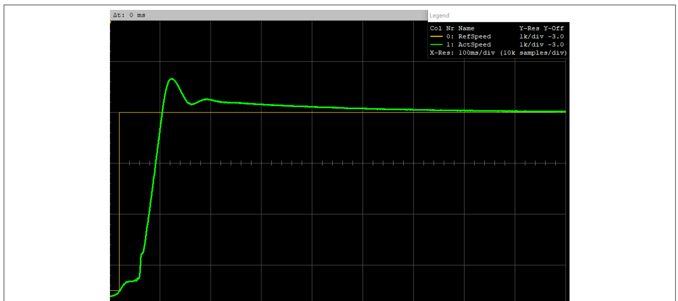
Figure 34 PI controller in time domain
