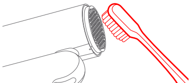
Cleaning Metal filter
