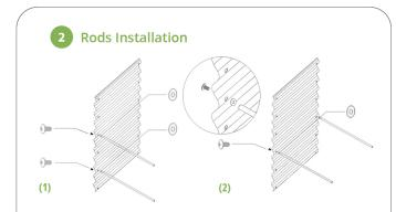
Install bracing rods between two parallel bolt holes. Attach bolt, panel, washer & rod loosely, connecting rods, then tighten them up with a screwdriver for reinforcement of the raised bed. (1) For 3.5ft wide configurations, the rods are installed in the **third** and **fifth** bolt holes from the top in the same row.
