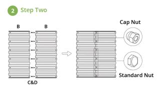
Cap nuts are used for top two rows, standard nuts are used for lower 4 rows. Assemble all straight panels: initially attach all bolts, washers and nuts loosely, and then tighten up using the wrench tool (as supplied) with a screwdriver/cordless drill.
