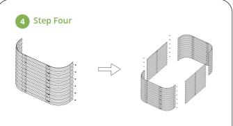
After straight panels are assembled, attach corner panels with straight panels using the same method. Make sure corner panels are attached outside of the straight panels.
