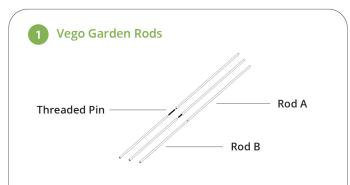
Vego Garden bracing rods are used to reinforce the strength of oversized raised beds. For 2ft wide raised beds: use A Rods only; For 3.5ft wide raised bed: use the threaded pins to connect A Rods to B Rods.
