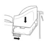
Place the battery door onto the bottom of the nozzle, slide it back into place and move the sliding tab next to the door to the lock position.
