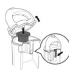
3 Press the top dust-cup release latch and pull up on handle. Lift out metal screen and clear debris.
