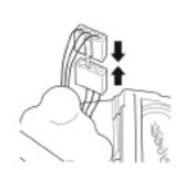
Push the connector terminals together until they lock into place.
