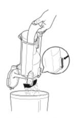
2 Hold dust cup over a trash bin and press the bottom dust-cup release latch.
