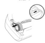
Once the brushroll has been cleaned, reinsert by slipping the black belt back onto the white gear.
