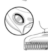
Press the power button once to turn on the carpet setting. The brushroll will spin quickly in this mode to get deep carpet cleaning.
