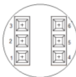
Figure 19. MEMS microphone coupon connectors CN25 and CN26 (top view)
