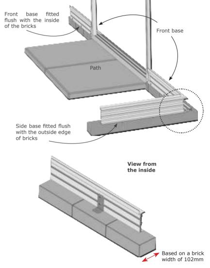
Greenhouses Direct RECOMMEND solid and flat engineering bricks to ensure a good anchor point
