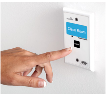
REMOTE STATION The Remote Station is a small, wireless RF device that can be mounted on a wall or other surface to send a preprogrammed response (e.g., identify room status as clean/dirty, call for vital signs, call for staff assist).
