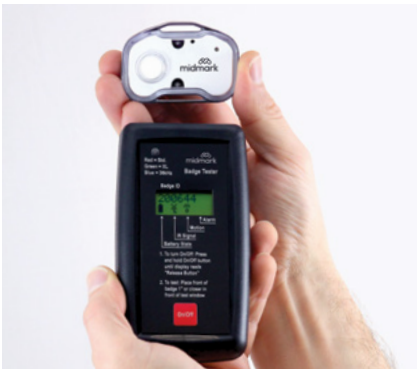
BADGE TESTER Check the status of IR badges or tags using our hand-held Badge Tester. The LCD screen shows a reading of badge/tag ID number, battery state, IR signal type, motion state and alarm state.
