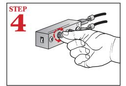
If necessary adjust the temperature by turning the adjustment stem clockwise to increase.
