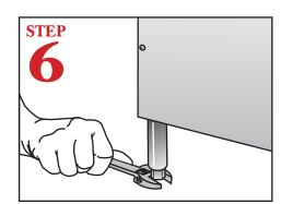
Level dishmachine by adjusting leveling legs. Dishmachine must be level front and back.
