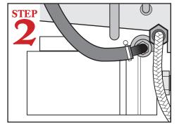
Connect dishmachine to hot water source 120°F - 140°F. Minimum temperature will remain in wash cycle until booster heater temperature reaches 180°F, then it will advance into rinse cycle.
