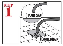
Connect the drain hose to floor drain. The floor drain must have a 1 inch air gap between drain hose and floor drain.
