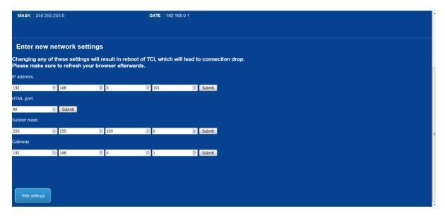
The Edit entry warns you if the number entered is incorrect. IP address entry is from 0 to 255 Port entry is from 0 to 65353
