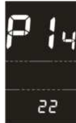
Current-limiting setting interface of the controller
