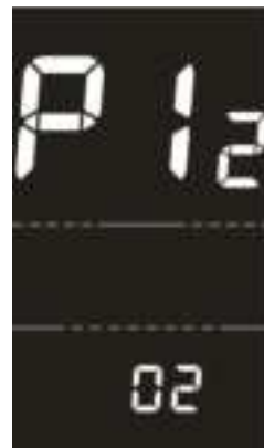
Power boost startup strength setting interface
