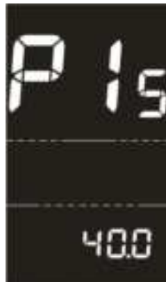
Battery undervoltage value setting interface
