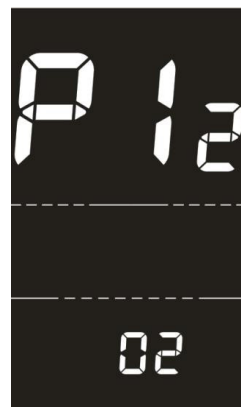
Power boost startup strength setting interface
