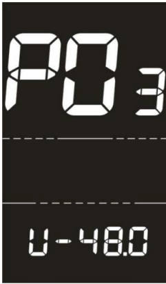
The rated voltage setting interface
