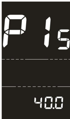
Battery undervoltage value setting interface
