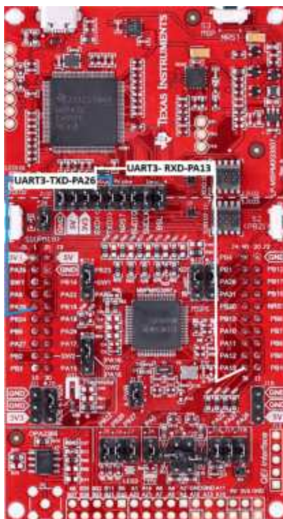
Figure 2-5. LP-MSPM0G3507 Backchannel Connection to UART3
