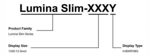
Figure 3-1 Naming rules for Lumina Slim-1330
