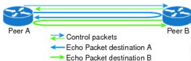
Figure 18: BFD Asynchronous Mode With Echo Packets
