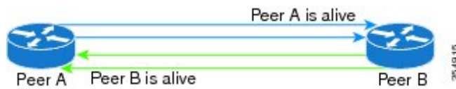
Figure 17: BFD Asynchronous Mode Without Echo Packets
