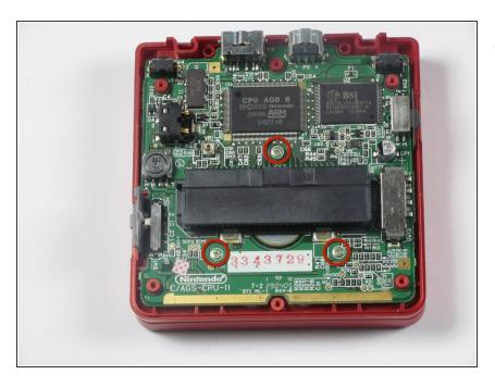
Using a Phillips #00 screwdriver, remove the three Phillips #00 4 mm long screws that hold the motherboard to the button panel.
