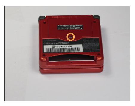
Use a standard Phillips #00 screwdriver to loosen the 4 mm screw that keeps the battery cover attached to the device.
