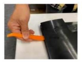
5. Use the Plastic Hera Jig to open the buckle on the bottom
