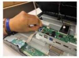
7. Disassemble the key board and speaker
