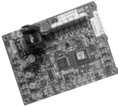
Figure C-1. ZN010 Control Board
