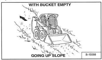
With an empty bucket, go down or up the slope with the heavy end toward the top of the slope [Figure OI-100] and [Figure OI-101].
