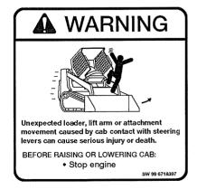
NOTE: On Advanced Control System (ACS) equipped machines, the steering levers could contact the cab frame while raising or lowering the operator cab. The engine MUST be stopped before raising or lowering the cab.
