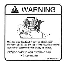
NOTE: On Advanced Control System (ACS) equipped machines, the steering levers could contact the cab frame while raising or lowering the operator cab. The engine MUST be stopped before raising or lowering the cab.
